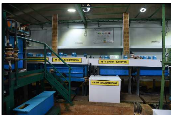
Fig. 7: Pilot scale facility for Gd oxide production at IREL
