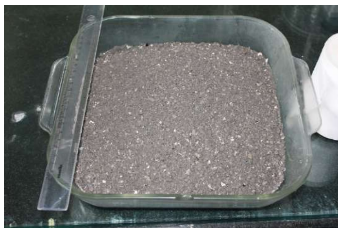
Fig. 11 NdFeB magnet powder after jaw crushing magnet (100 pieces)
