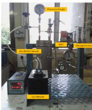
Figure7: Experimental setup for breakthrough studies with packing material
