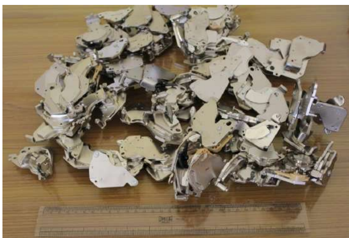
Fig. 10: NdFeB magnets recovered from EOL computer hard disk drives
