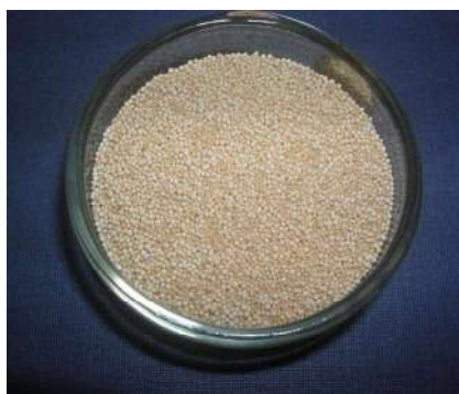
Figure 9: Novel chemical adsorbent for CO 2 adsorption (left). Dimensionless CO 2 concentration versus time at 30°C (right)
