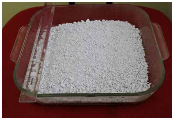
Fig. 12: Rare earth oxide separated from NdFeB magnet scrap
