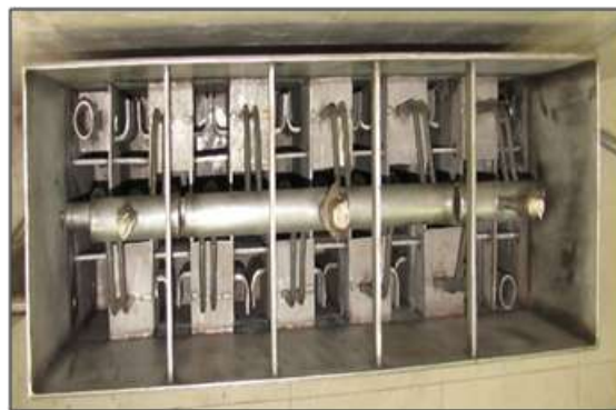
Fig.6 : (a) Actinide separation demonstration facility, Tarapur (b) Air lift-based mixer settler unit utilized for the partitioning of HLW
