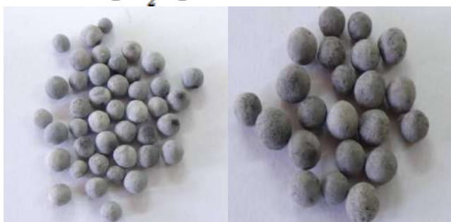
Figure 6: Palladium (0.5% & 1.0%) on Alumina Catalyst developed by BARC
