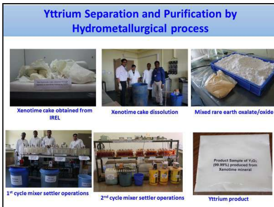
Fig. 4: Xenotime feed source, 1 st & 2 nd cycle SX set up, mixed product obtained in 1 st cycle, high pure Y product from complex HRE mineral Xenotime: process demonstration to IREL personnel
