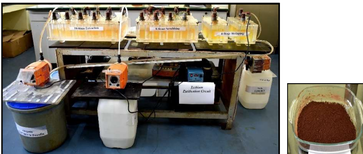
Fig. 9: Counter current SX process for Tb purification and \text{Tb}_4\text{O}_7 (>99%) product
