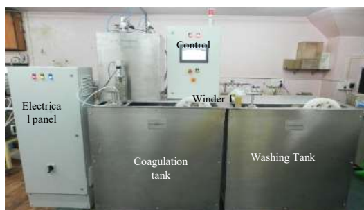
Figure 21: Hollow fibre membrane spinning machine
